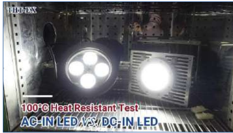
100°Cの高温環境での比較 AC-IN LED vs. DC-IN LED
